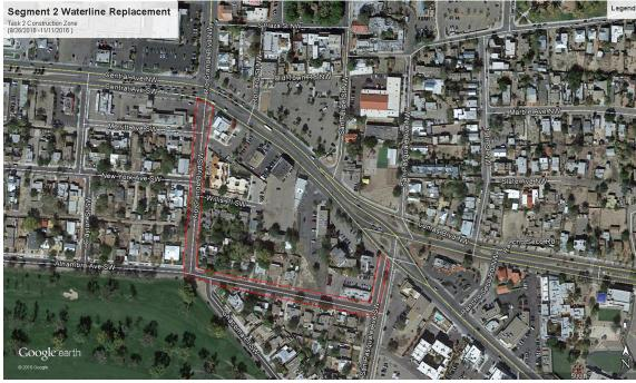
Crews will be installing a new 16" water line that will be replacing a 16" water line that runs from Rio Grande to San Pasqual in Central Ave. The old 16" water line in Central will be grout filled and abandoned in place. As part of this work, an old 6" line
